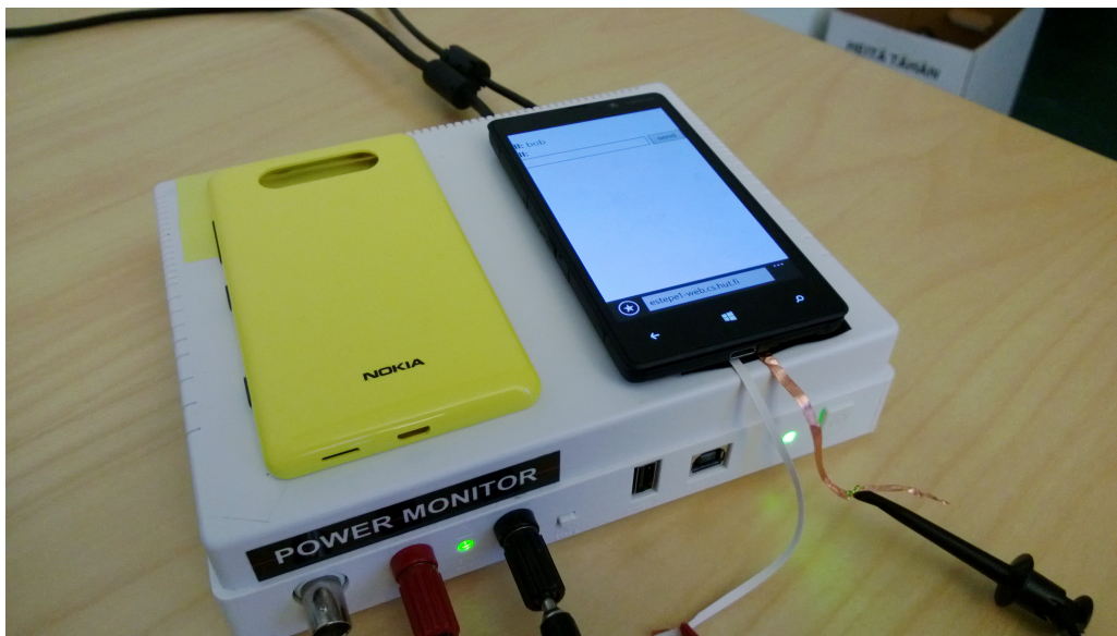
Figure 5.2: Nokia Lumia 820 connected to Monsoon Power Monitor.
